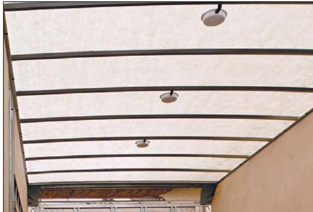
Translucent roof shown with (2) additional domelights
