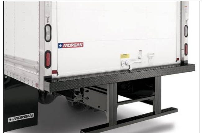
Various bumpers and under-ride configurations
