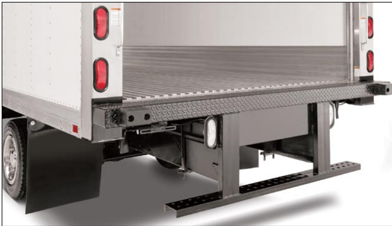
Various bumpers and under-ride configurations
