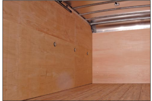
Plywood interior liner, shown with tie rings
